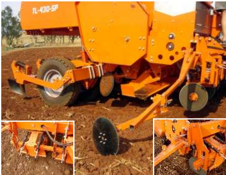
situated directly behind the furrow openers, thus allowing for immediate covering over of the planted seed to help eliminate the seed rotting due to being covered over with warm earth.
